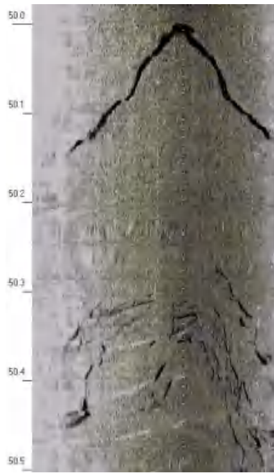
图8.3-7 50.0~50.5/40.96m深处斜交和垂向裂隙 图8.3-8 56.3/46.1m深处斜交和垂向裂隙
