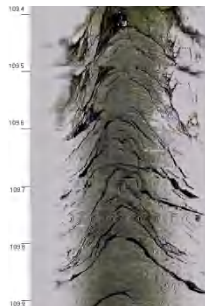
图8.3-14 109.4~109.9/89.62m深处横向裂隙
